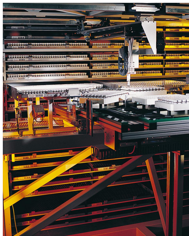
Figure 2. The Haystack system (The Automation Partnership) allows a compound library to be managed and dispensed from solid or liquid archives.
