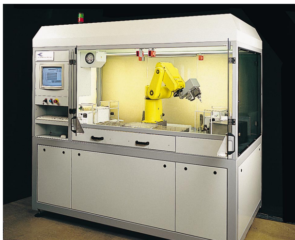
Figure 3. The robotic arm of the Haywain (The Automation Partnership) feeds sample vials to the balances ensuring that they are never standing idle.
